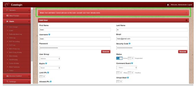
**Step 1.** Check if the user exists on the gateway server by finger or id command.
