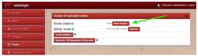
Step 3: Then remove the other node by Web Panel > Cluster > "Remove" button for "Other Node"
