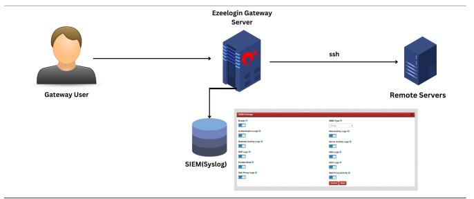
Step 1: Login to Web GUI and navigate to Settings - > SIEM -> SIEM type to syslog and enable logs.
