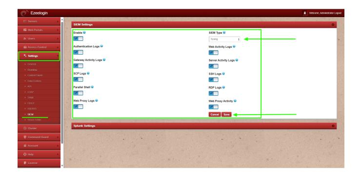
By enabling this feature, all active logs will be directed to the syslog of the gateway server. You can monitor these logs by tailing the syslog and executing the SIEM script in a separate shell to analyze the forwarded logs.
