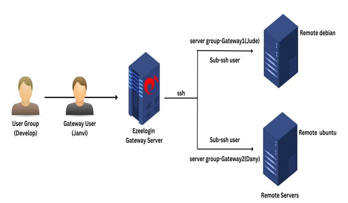
Ssh-user logs into different remote servers with different sub-ssh accounts.
