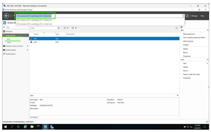
Paste the distinguish name in Base DN field and paste in LDAP settings in Ezeelogin GUI.
