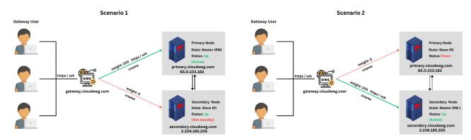
Scenario 1: **Primary node is in active state and secondary is in the hot standby mode**. Traffic is routed to the primary node.
