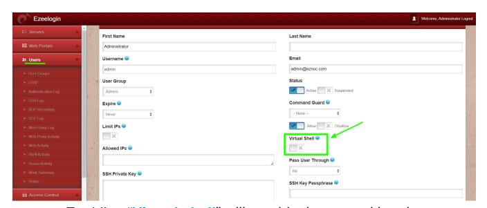
**Step 2:** Enabling "Virutal shell" will provide the user with only a non-interactive shell that just lets gateway users to execute commands on the remote server (similar to parallel shell) with complete **command** guard filtering capabilities.
